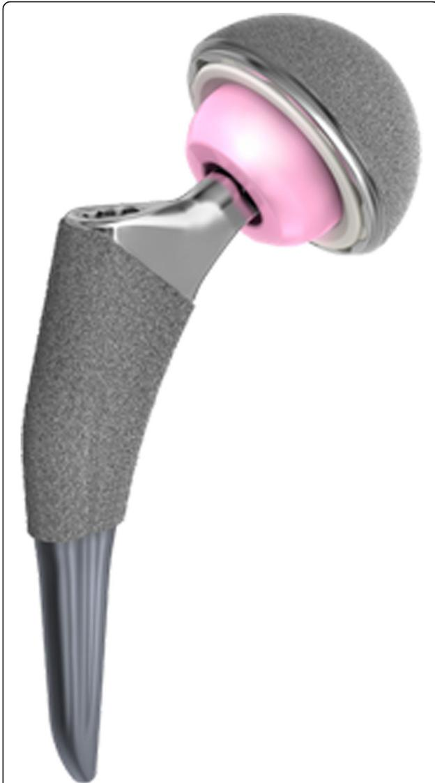
**Fig. 2** The type-4 stems are rarely neck-preserving and often extend to the upper diaphysis. With their tapered-wedge design and proximal porous coating, they achieve fixation proximally. These are similar to conventional, proximally porous-coated tapered designs with a shorter length or reduced distal end of the stem
