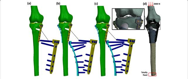
Fig. 2 Fixation strategies and bonudary condition used in this study, including a MP, b BP without D-hole screw, c BP, and d boundary condition
