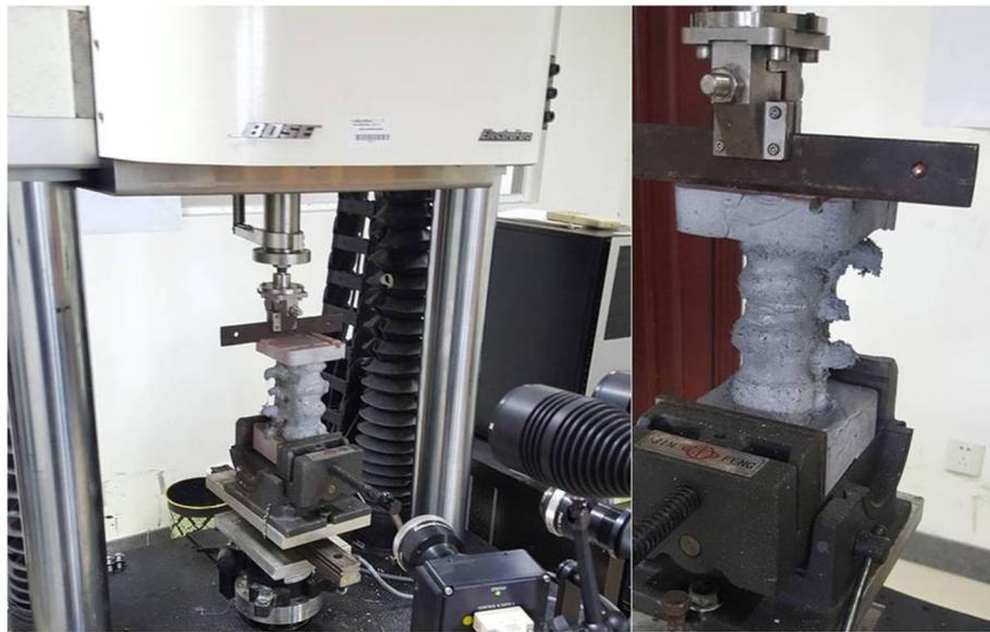
**Fig. 2** Specimens were placed on the mechanical test machine for testing
