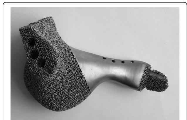
**Fig. 6** Posterior view of the endoprosthesis fabricated by electron beam melting technique. The porosity was 70% and pore size was 600  $\mu\text{m}$
