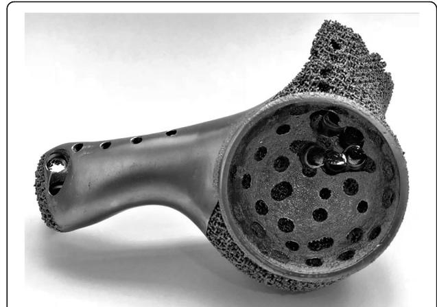
**Fig. 5** Anterior view of the endoprosthesis fabricated by electron beam melting technique. The porosity was 70% and pore size was 600  $\mu\text{m}$
