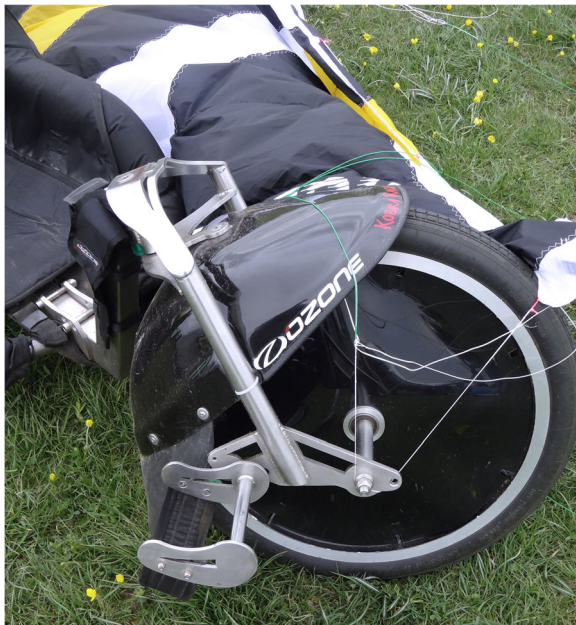
Fig. 2 Straps attached to the front wheel allow the kiter to steer the buggy
