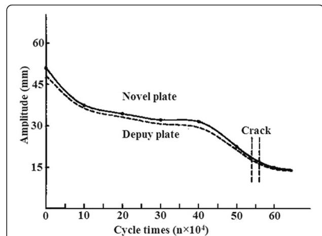
**Figure 4** The fatigue life curves for the novel plate and the DePuy plate.
