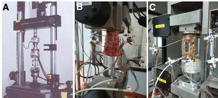
**Figure 3 Experimental setup.** (A) The composite MTS 858 biomechanical testing machine and the test sample. The range of motion, load-displacement, torque, and twisting stiffness tests for the normal specimens (B) and the novel self-locking plate fixed specimens (C).
