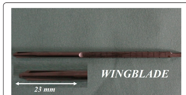
Figure 1 The wingblade of the torque measurement device (DensiProbe Hip™) had a diameter of 6.5 mm and a length of 23 mm.
