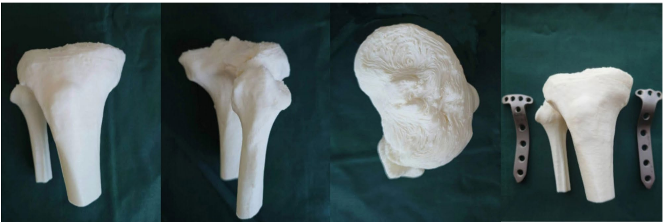
Fig. 4 3D printing of the physical model of the fracture after encoding the fracture fragments
