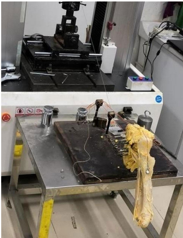
Fig. 1 The customized equipment consisted of a baseplate and several pulleys for changing the direction of the steel wire, the steel wire connects the deltoid tubercle and the actuator
