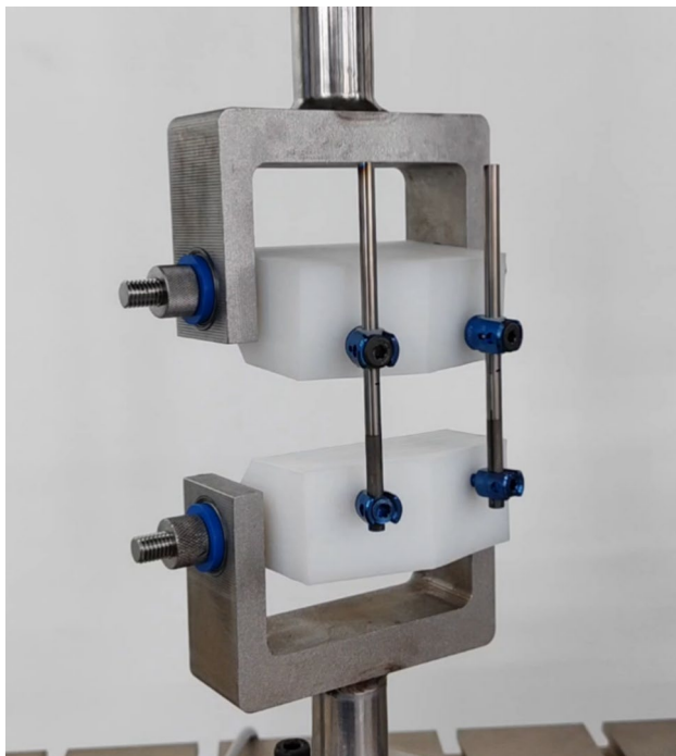
Fig. 2 The sample of the novel growth guidance system installed on the MTS test system. The novel growth guidance system (4.5-mm system) was installed on the simulated vertebrae (UHMWPE module) and tested by MTS test system. The sliding poly-axial pedicle screws were placed on the upper simulated vertebra and captured polished parts of the rods with the UHMWPE gaskets. The fixed-head pedicle screws were placed on the lower simulated vertebra and locked un-polished part of the rods
