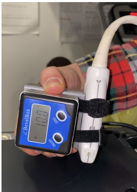
Fig. 3 Digital inclinometer housed within a 3D-printed case affixed to the US transducer with Velcro straps
