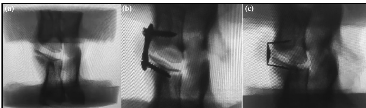
Fig. 3 a, b, c Radiographs of specimens before internal fixation and after performing different internal fixations
