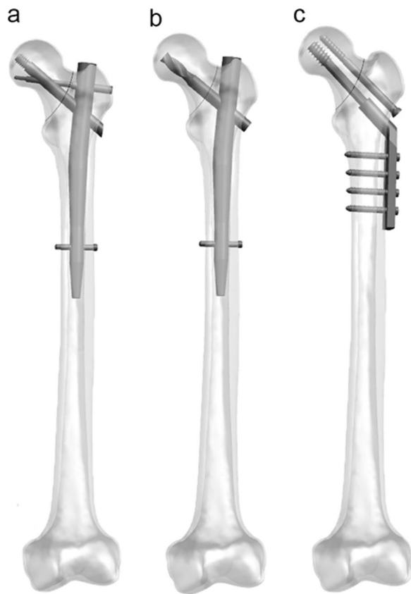
Fig. 1 The femur model with three types of implants: a proximal femoral bionic nail (PFBN), b proximal femoral nail anti-rotation (PFNA) and c dynamic hip screws with de-rotation screw (DHS + DS)
