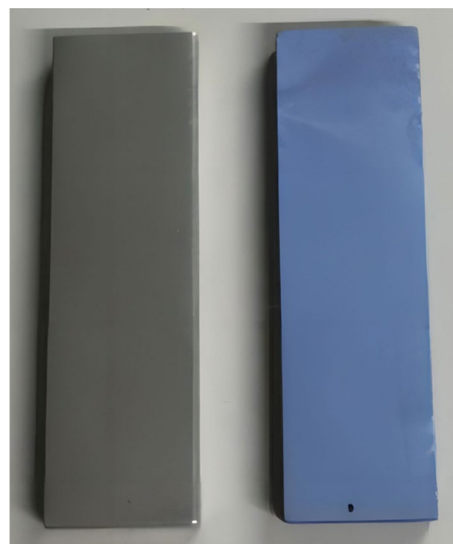
Fig. 2 Visual characteristics of the titanium plate. The titanium plate after grinding and pretreatment (left) and the titanium plate bearing TiO 2 nanotubes after anodization (right)
