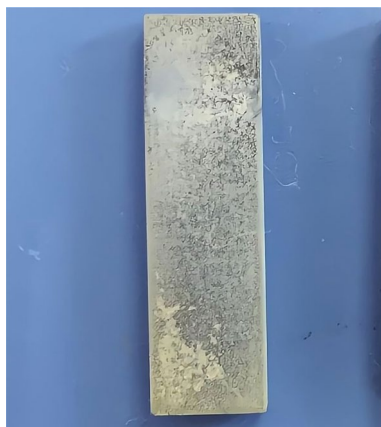
Fig. 4 Visual characteristics of iodine-doped TiO 2 nanotube-coated titanium plate. Appearance of the iodine-doped TiO 2 nanotube-coated titanium plate. After the electrophoretic deposition of iodine onto the TiO 2 nanotube arrays, a light-yellow granular coating was observed on the surface of the titanium plate
