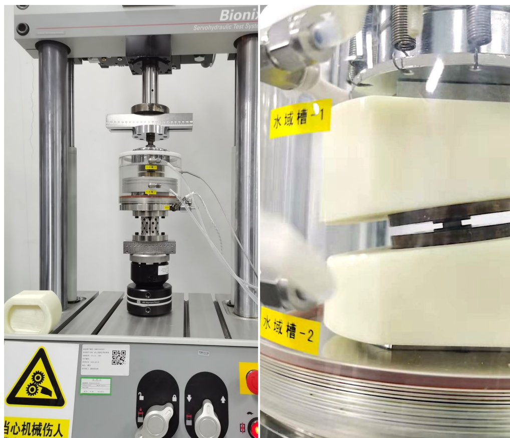
Fig. 3 The creeping test was performed on a biaxial servo-hydraulic testing machine MTS Mini Bionix II 858 (MTS Systems Corp., USA) with 3600 N load for 24 h
