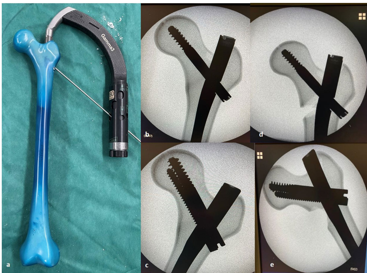
Fig. 1 a The instrumentation of Gamma3 has been applied in a standard manner, according to the manufacturer's manual in an osteoporotic Sawbone model, first on the intact sawbones; b–d Fluoroscopic images of Gamma3 in the intact and fractured Sawbone; c–e Fluoroscopic images of InterTan in the intact and fractured Sawbone
