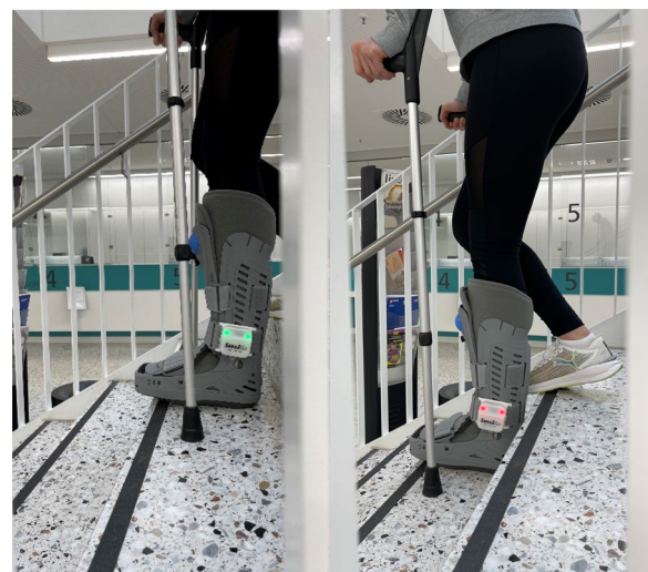
Fig. 1 Loads under 20 kg results in a green light (left), over 20 kg in a red light accompanied by an audible "beep"-sound (right)
