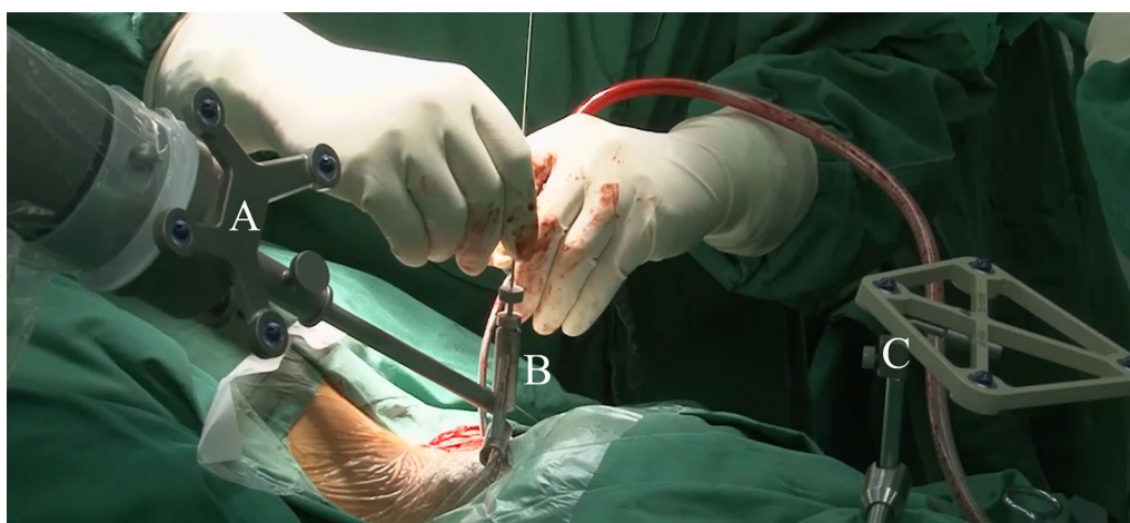
Fig. 3 Intraoperative instrumentation. A The robot arm with a tracker; B The guider with the guiding tube inside; C The patient tracker attached to the Mayfield frame
