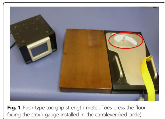
**Fig. 1** Push-type toe-grip strength meter. Toes press the floor, facing the strain gauge installed in the cantilever (red circle)
