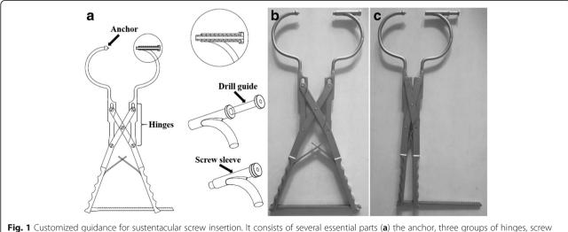
**Fig. 1** Customized guidance for sustentacular screw insertion. It consists of several essential parts (**a**) the anchor, three groups of hinges, screw sleeve, drill guide, and two clamp arms. The two arms of the clamp are combined through three groups of hinges. The drill guide is removable while the screw sleeve is fixed. The entry and exit of the screw sleeve are always in line with the anchor during opening (**b**) and closing (**c**) of the device
