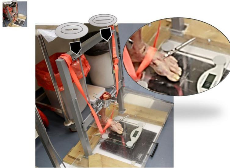
**Fig. 3** The forefoot was mounted on a scale at 15° tilt and restrained by straps. Weights were added until the scale showed the desired weight (original weight of the specimen donor). *Arrows* represent the weights which are added and placed on the top of the construct
