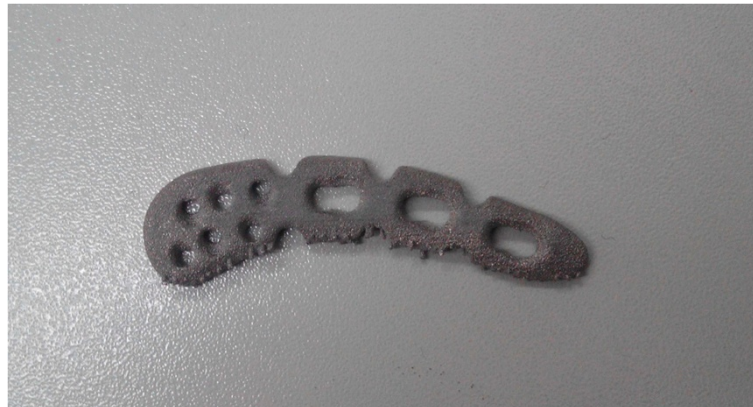
Figure 1 The EBM-printed Ti-6Al-4V LCP plate.
