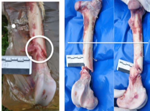
Figure 2 Representative photographs of the thigh-shaped gelatine sample, which produced a remote fracture. On the left is the embedded femur being dissected with the bullet path shown as a dot and the fracture circled. On the right are an anterior and a medial view of the dissected fracture with a line representing the height of the bullet on the bone.
