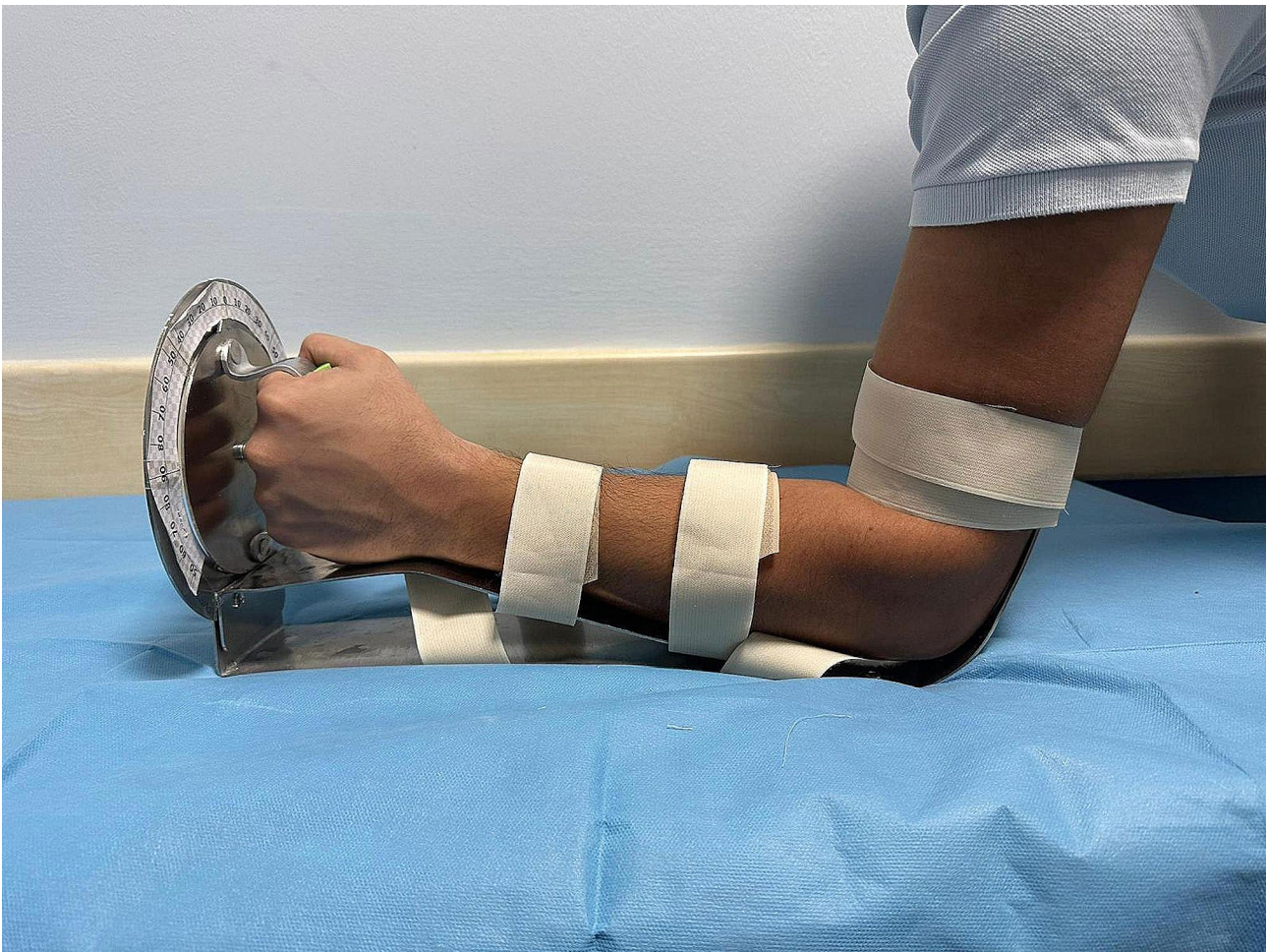
Fig. 1 Custom-made goniometer. A circular goniometer is attached vertically to platform and grabbed by a handle. Forearm and arm fixed with help of bandages while elbow is at 90 degrees
