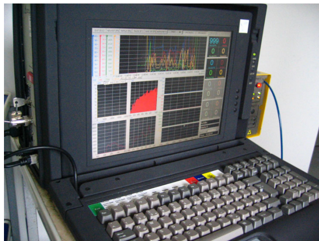
Figure 2 Oxygen-to-see system combining Laser Doppler flowmetry and spectrophotometry non-invasively to determine tendon capillary blood flow, tendon oxygen saturation, and tendon postcapillary venous filling pressures.
