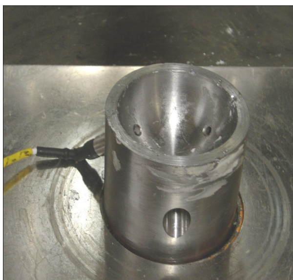
Figure 1 Metal acetabulum with a transducer.
